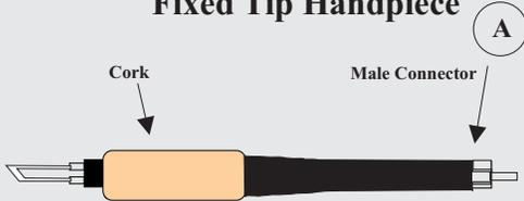
The Fixed Tip handpiece and the RT handle connect to the Handpiece cord in exactly the same manner; Male Connector inserts into the Female connector. The burning tip cannot be removed from the Fixed Tip Handpiece.
